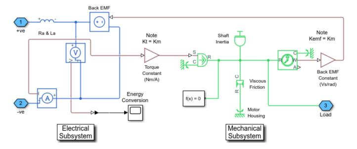
The DC motor model shows a relationship from current to torque (the green line on the left). The torque causes the shaft of the motor to spin and we have a relationship between this spinning to the Back EMF (electromotive force). The rest of the parameters include a shaft inertia, viscous friction (damping), armature resistance, and armature inductance.
