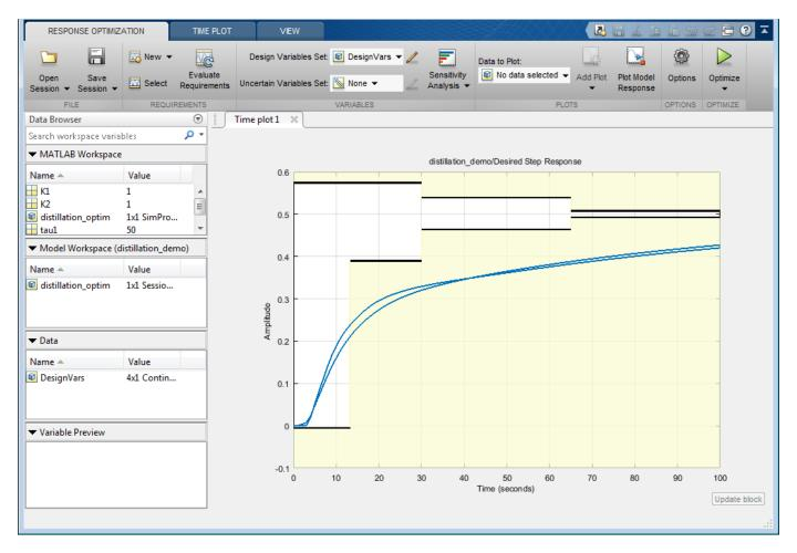
There are two curves in the plot representing the methanol composition in the top and bottom of the column.
