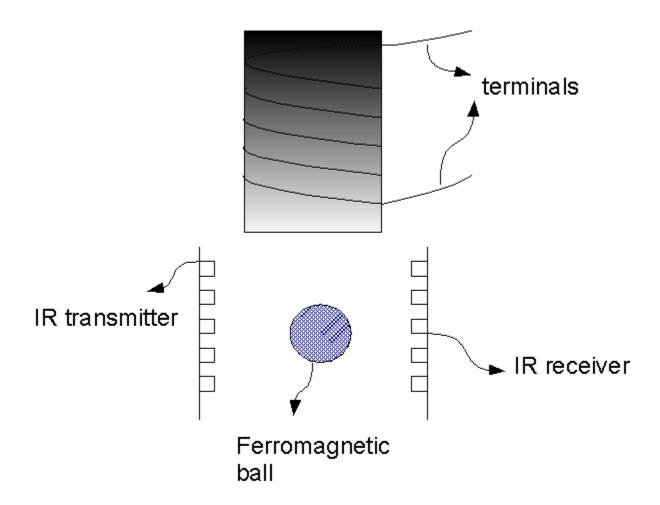
The physical system consists of a ball (with mass 0.00837 kg) which is under the influence of three forces:
