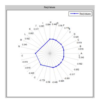
The plot has an axis for each edge-and-signal combination defined in the distillation\_demo/Desired Step Response check block. Points on each axis represent the violation for that signal-edge combination and the plot connects these points to form a closed polygon representing the initial design. Note that some points are negative, representing satisfied constraints, and some positive, representing violated constraints.
