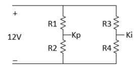
The proportional gain, Kp, is given by 12\*R2/(R1+R2) and the integral gain, Ki, is given by 12\*R4/(R3+R4). The initial values of the resistances are R1 = 47 k $\Omega$ , R2 = 180 k $\Omega$ , R3 = 10 k $\Omega$ , and R4 = 10 k $\Omega$ .
