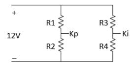
The resistances R1 through R4 are 47 kOhm, 180 kOhm, 10 kOhm and 10 kOhm respectively. These were chosen to set Kp and Ki to values that enable the controller to meet the requirements for
