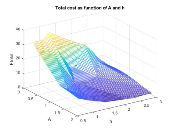
The plot shows that high values of A and h result in lower costs. The best design in the sampled space corresponds to the design with the lowest cost value.
