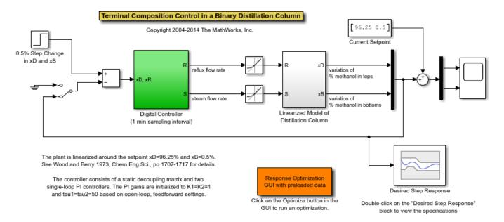
Double-click the Scope block to view the unoptimized methanol composition in the top and bottom of the column.
