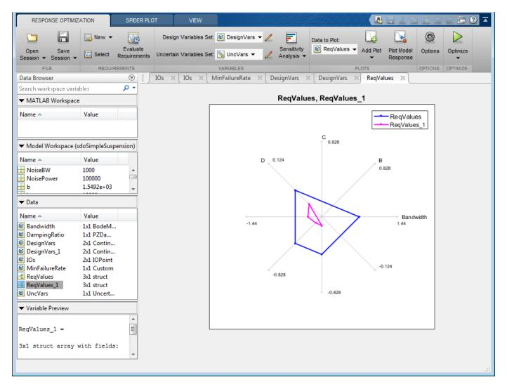
The plot shows that the optimal design has a lower failure rate (the MinFailureRate axis) and better satisfies the bandwidth requirement. The value plotted on the bandwidth axis is the difference between the bandwidth bound and the bandwidth value. The optimization satisfies the bound by keeping this value negative; a more negative value indicates better satisfaction of the bound.
