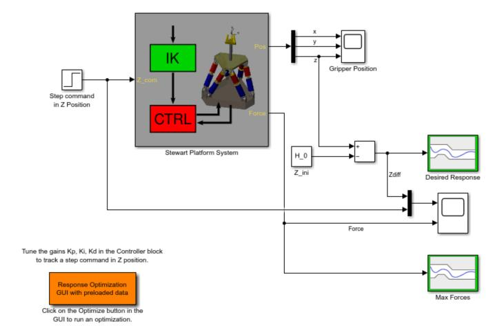
Double-click the Scope block to view the unoptimized position, the step input, and the controller's force actuation signal.
