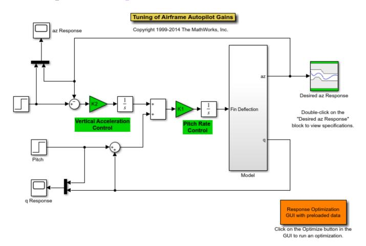
Double-click the az Response Scope block to view the unoptimized vertical acceleration az of the airframe.
