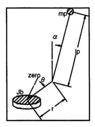
The system is modeled using Simscape Multibody. There are two bodies modeled in this system. The machine consists of one body representing the rotational arm and the other representing the pendulum. The bodies are connected by revolute joints that constrain the motion of the bodies relative to each other. An input voltage is delivered to a DC motor that provides the torque to the rotational arm.
