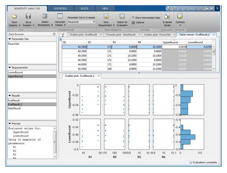
The **Sensitivity Analyzer** was used to explore the effect of standard precision components on the design requirements of a PI controller. With standard precision components, some requirements were found to be violated. Statistical analysis was used to identify which parameters most influence the requirements. The analysis resulted in replacement of only two of the four components with most costly high-precision components.
