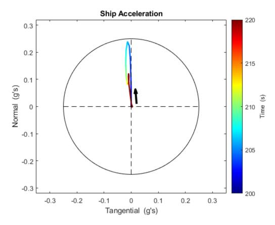
In this example, the ship plant varied with the ship speed, so the controller gains also needed to vary. Gain scheduling was implemented using lookup tables. By tuning the gains and breakpoint values in the controller, the ship was able to follow the reference heading angle, while also constraining total acceleration to ensure a safe and comfortable ride for passengers.
