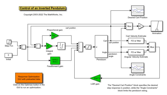
Double-click the Desired Cart Position block to view constraints on the cart position of the inverted pendulum.
