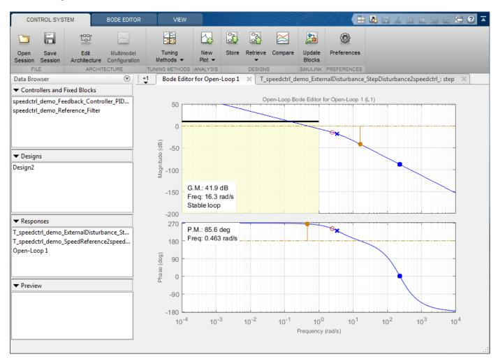
Add **Requirement 4** for the maximum loop gain to the Bode magnitude plot to satisfy the overall design specifications. The Bode magnitude plot shows the minimum and maximum loop gain over the specified frequency range.
