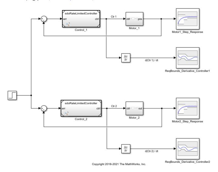
Two motors are controlled. Model references are used for the controllers, which are instances of the same model. Open the controller.
