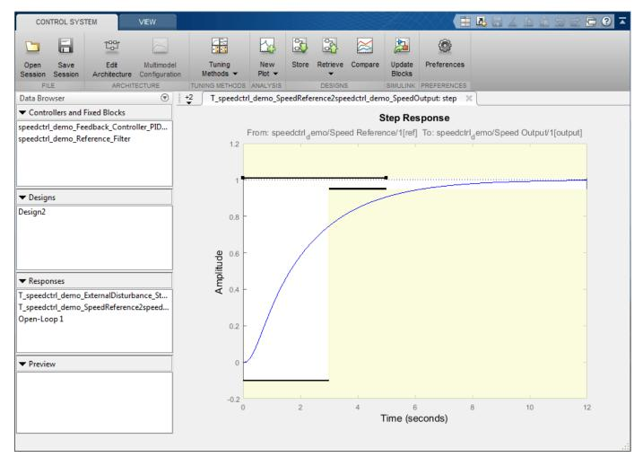
The plot shows the lower amplitude limit of -0.1, maximum overshoot and 95% of the unit step response value of 1.01 and 0.95 respectively.
