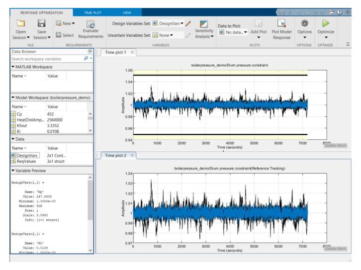
The final response shows that the optimized regulator tracks the reference pressure much more closely and the drum pressure constraints are satisfied.
