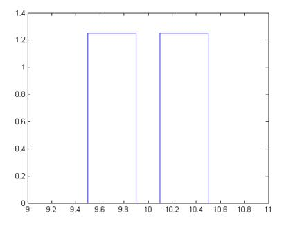
makedist specifies a piecewise linear distribution for the resistor value, with a "hole" in the 1% range.
