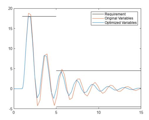
Now the motor position is within the spec of the disturbance rejection requirement.
