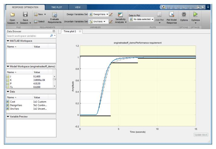
The optimization project saved with the example corresponds to stage 2. In this stage, we optimize the controller parameters over the operating range. To do so, we specify K, P and Z as tuned parameters and the final step value, final\_step, of the reference signal as an uncertain parameter. At this stage, the custom controller cost objective is not included in the optimization problem.
