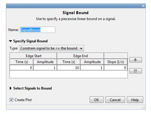
Designate the **Requirement Name** as MaxPressure. In both the start and end **Amplitude** columns, enter the maximum pressure requirement of 1.75e6 N/m, and set the **Edge End Time** to 0.1 s. In the **Select Signals to Bound** area, select Pressures, the signal on which this requirement applies.
