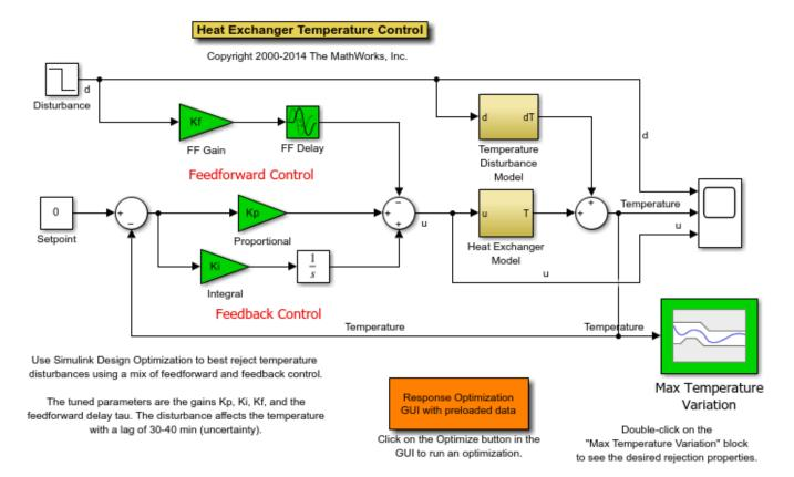
Double-click the Scope block to view the unoptimized temperature response, the disturbance signal and the control signal.
