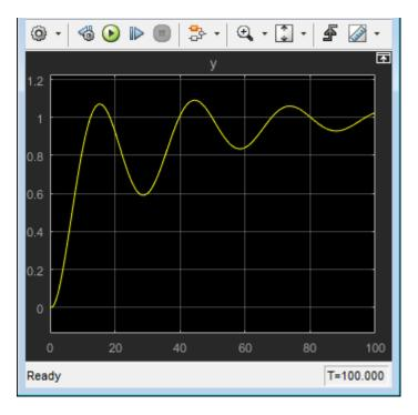
Double-click the Step Response Specifications block to view constraints on the plant response, including rise time, settling time and maximum overshoot.
