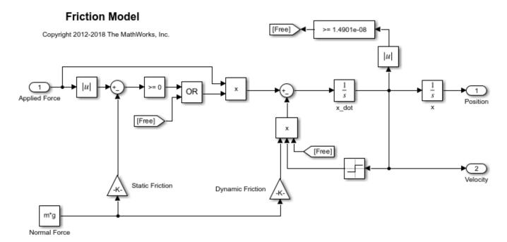
The model is based on a mass sliding on a surface. The mass is subject to a static friction that must be overcome before the mass moves and a dynamic friction once the mass moves. The static friction,  $u_static$ , is a fraction of the mass normal force; similarly the dynamic friction,  $u_dynamic$ , is a fraction of the mass normal force.
