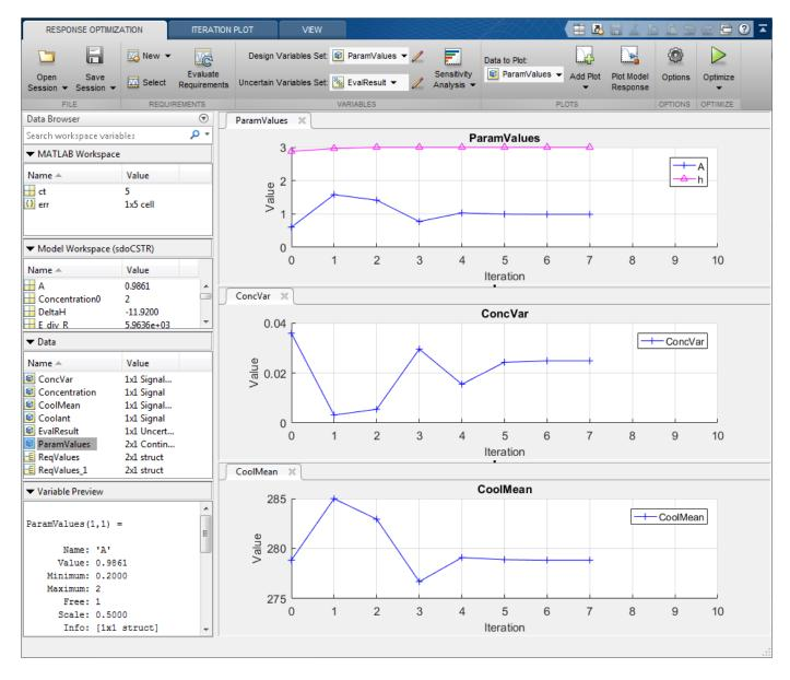
The optimization minimizes CoolMean and ConcVar in the presence of varying FeedCon0 and FeedTemp0.
