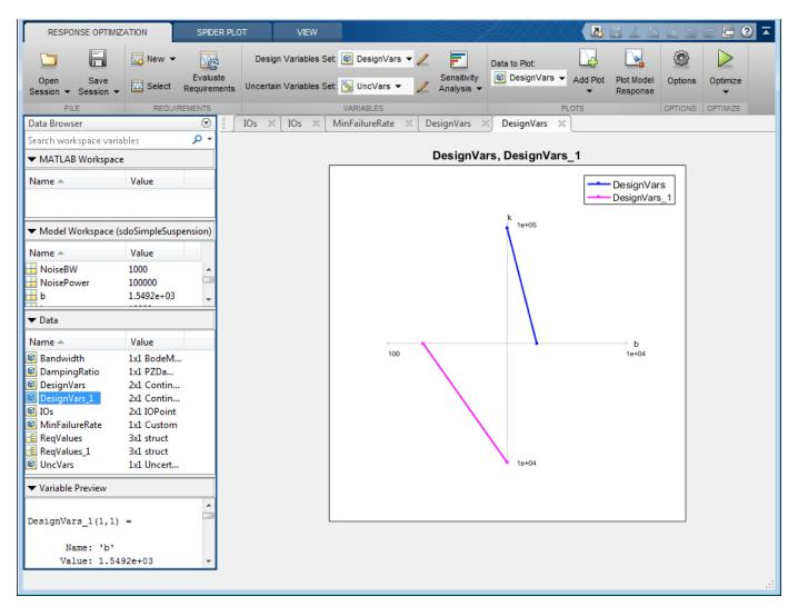
The plot shows that the optimizer reduced both the k and b values for the optimal design.
