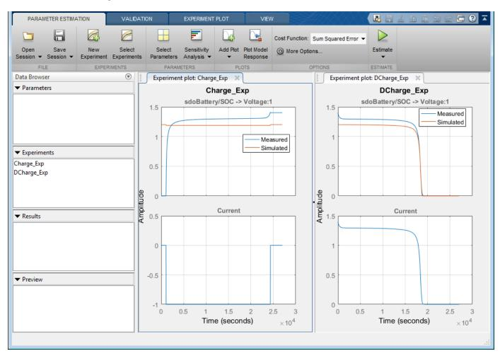
The plots show that the battery initial charge Q0 is not set correctly for the Charge\_Exp experiment and that the model V, K, and Loss parameters need to be estimated.
