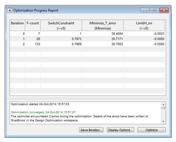
The Optimization Progress window appears and updates at each iteration. The optimization successfully minimizes the temperature error while satisfying the switching constraints.
