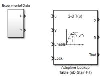
Assign the input and output data to the engine model by connecting the U and Y ports of the Experimental Data block to the u and y ports of the Adaptive Lookup Table block, respectively.
