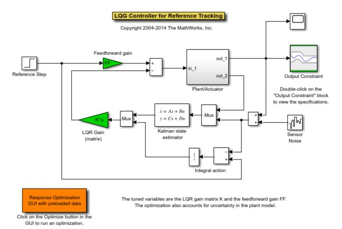
Double-click the Plant/Actuator block to view the details of the subsystem. Note that the plant is represented in State-Space form in this model and includes Rate Limiter and Saturation blocks.
