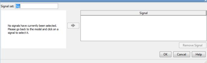
Enter Pressures as the signal name in the **Signal set** field. Then, in the Simulink model, click the first output port of the Cylinder Assembly block named Pressure. The dialog updates to display the selected signal.
