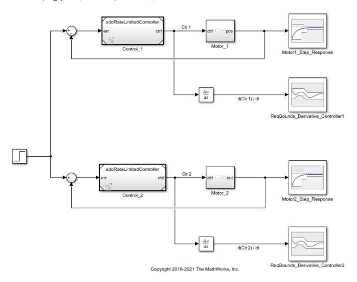
Model references are used for the two controllers, which are instances of the same model. Open the controller.
