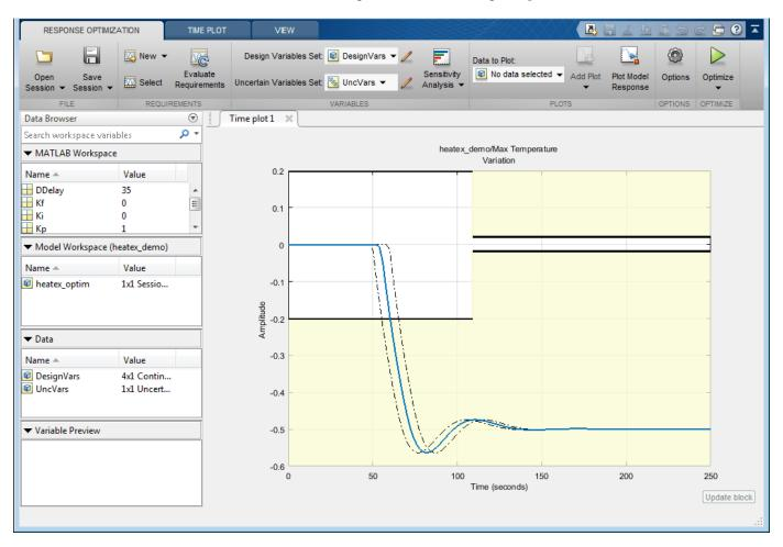
The solid line represents the current response with the mean Disturbance Delay as specified in the constraint block. The dashed lines represent the response with the maximum and minimum Disturbance Delay.
