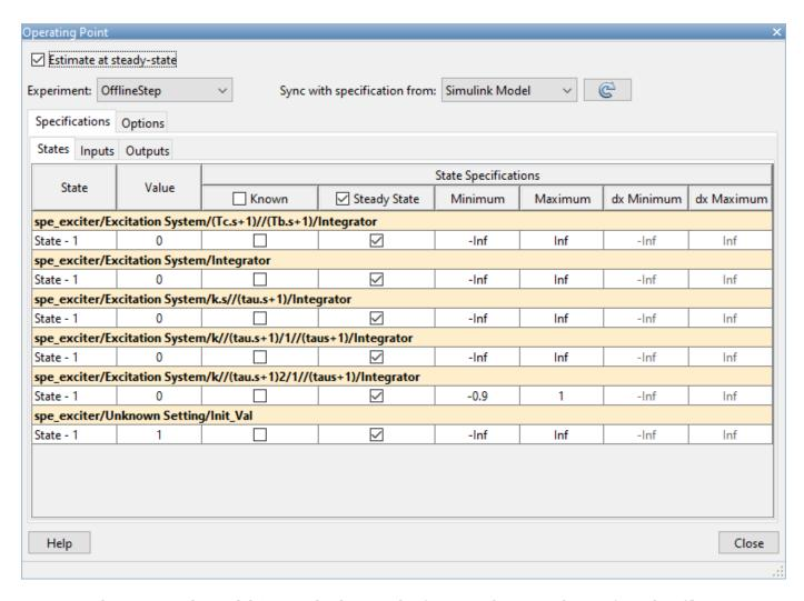
The inputs to the model (terminal voltage and reference voltage) are known from the offline step test. Switching to the **Inputs** tab under **Specifications**, we can specify these conditions. We can see that the inputs are marked as known by default with a value of one. These come from the starting value in the measured data, and we will leave these values unchanged.
