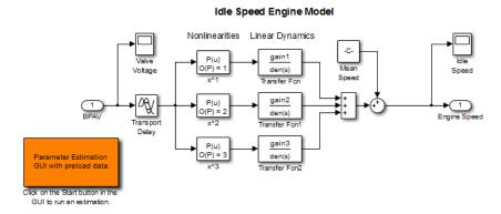
The model contains the Inport block BPAV and Outport block Engine Speed for importing input and output data, respectively. To learn more, see "Model Requirements for Importing Data" on page 1-2.
