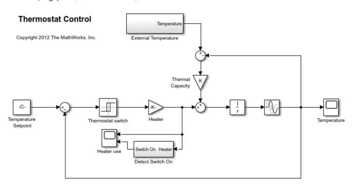
The model describes a simple heater & thermostat that regulate the temperature of a room. The room is subject to external temperature fluctuations. The room temperature is computed using a first-order heat-flow equation:
