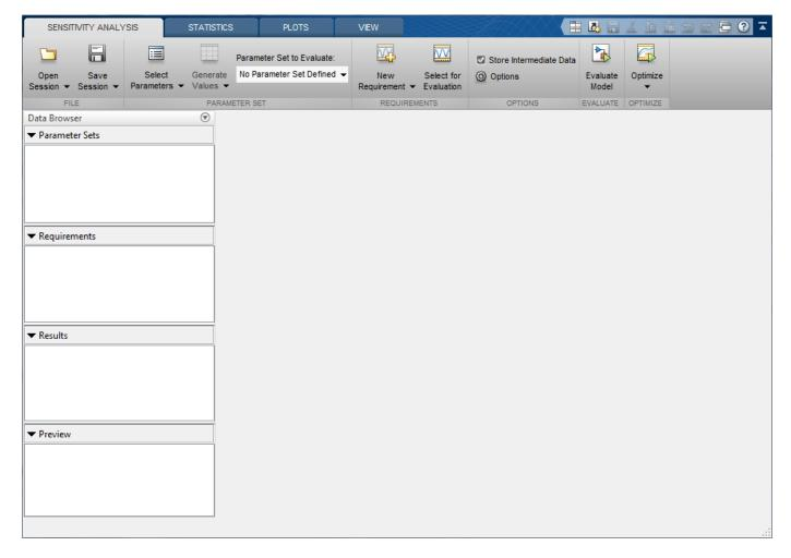
Create a parameter set that includes the CSTR design variables A and h and the feed variation parameters FeedConc0 and FeedTemp0. You randomly generate multiple values for these parameters to evaluate the CSTR design.
