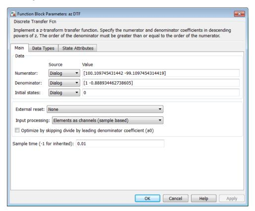
Mask of a Simulink Compensator Block
